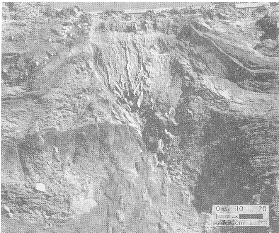
Plate 1. Vertical lineations in sand wedge. Lineations stand out in relief due to weathering of section. Notice the upturned beds surrounding the wedge
